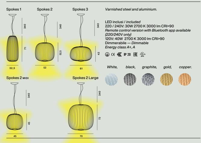
Light volumes that contain light and at the same time allow it to flow into space. The double LED source lights the surface below perfectly, while creating magical games of light and shadow on the walls and ceiling.
